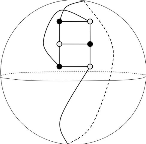
Figure 3: An attempt to draw  $K_{3,3}$  on the sphere. Dashed lines indicate edges that go along the back of the sphere. Notice that the long edge being sent behind the sphere still cuts the space into two halves, and the remaining edge is forced then to cross the line in order to connect the two vertices from the two halves.
