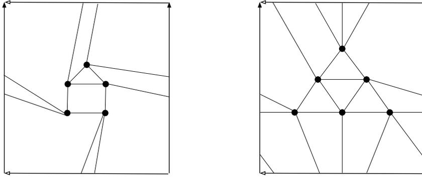
Figure 8: Two graphs embedded on the torus. The astute observer will recognize these as the complete graphs on 5 and 6 vertices, respectively, neither of which can be embedded into the plane.
