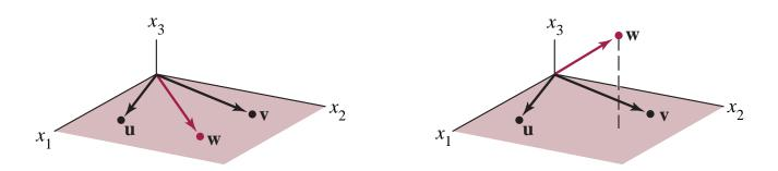
Linearly dependent, w in Span{u, v}
