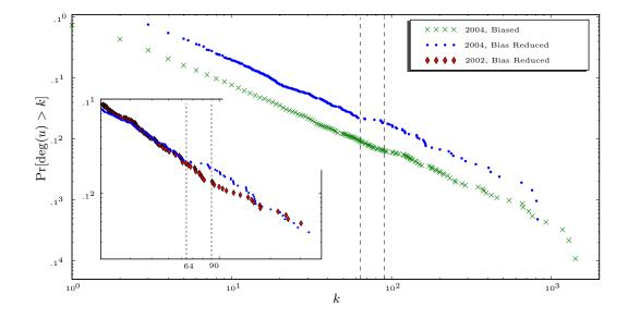
Fig. 1. Degree sequence ccdf estimates for the AS graph (from CAIDA skitter). Main panel: March, 2004, with and without bias reduction. Inset: a portion of ccdf for March, 2004 and March, 2002, both with bias reduction. The nodes with degree between 65 and 90 in 2002 have disappeared in 2004.
