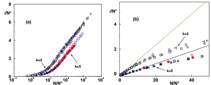
FIG. 17. Data collapse  $\ell(N, p)/N^*(p)$  versus  $N/N^*(p)$  for two different values of  $K$ . (a) Log-linear scale showing the logarithmic behavior at large  $N/N^*$ ; (b) Linear scale showing the linear behavior  $\ell(N, p) \sim N/(4K)$  at small  $N/N^*$ . After Barrat and Weigt (2000).
