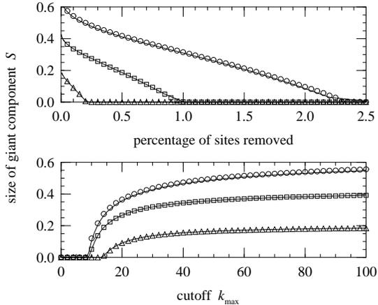
FIG. 34. Fraction of nodes in the spanning cluster in scale-free random networks with all nodes with degree greater than  $k_{max}$  unoccupied, for  $\gamma = 2.4$  (circles),  $\gamma = 2.7$  (squares) and  $\gamma = 3.0$  (triangles). The solid lines are the analytical prediction. Upper frame: as a function of  $f$ . Lower frame: as a function of the cutoff  $k_{max}$ . After Callaway *et al.* 2000.
