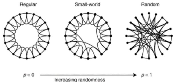
FIG. 15. The random rewiring procedure of the WS model which interpolates between a regular ring lattice and a random network without altering the number of nodes or edges. We start with  $N = 20$  nodes, each connected to its 4 nearest neighbors. For  $p = 0$  the original ring is unchanged; as  $p$  increases the network becomes increasingly disordered until for  $p = 1$  all edges are rewired randomly. After Watts and Strogatz (1998).
