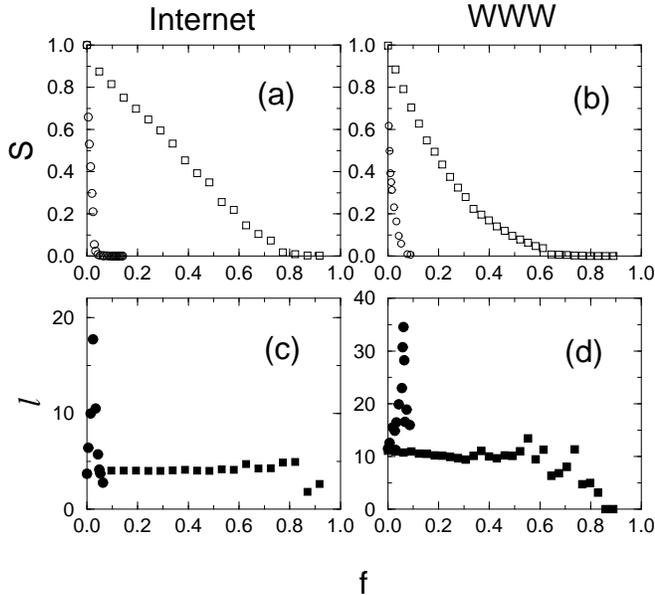
FIG. 35. The relative size  $S$  (a, b) and average path length  $\ell$  (c, d) of the largest cluster in two communication networks when a fraction  $f$  of the nodes are removed. (a, c), Internet at the domain level,  $N = 6,209$ ,  $\langle k \rangle = 3.93$ . (b, d) Subset of the WWW with  $N = 325,729$  and  $\langle k \rangle = 4.59$ . Squares indicate random node removal, circles mean preferential removal of the most connected nodes. After Albert, Jeong, Barabási 2000.
