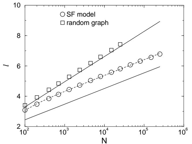
FIG. 23. Characteristic path length  $\ell$  versus network size  $N$  in a network with  $\langle k \rangle = 4$  generated by the SF model (circles), compared with a random graph with the same size and average degree generated with the algorithm described in Sect. III.A (squares). The dashed line follows Eq. (93), and the solid lines represent Eq. [59] with  $z_1 = \langle k \rangle$  and  $z_2$  the numerically obtained number of second neighbors in the respective networks.
