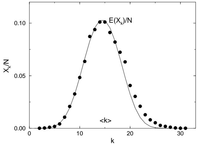
FIG. 7. The degree distribution that results from the numerical simulation of a random graph. We generated a single random graph with  $N = 10,000$  nodes and connection probability  $p = 0.0015$ , and calculated the number of nodes with degree  $k$ ,  $X_k$ . The plot compares  $X_k/N$  with the expectation value of the Poisson distribution (13),  $E(X_k)/N = P(k_i = k)$ , and we can see that the deviation is small.
