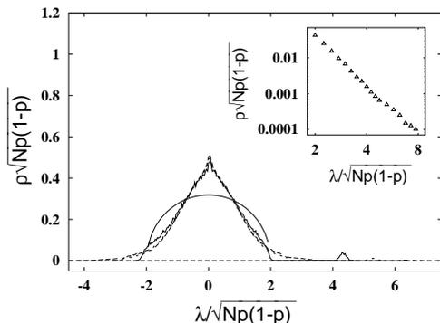
FIG. 25. Rescaled spectral density of three networks generated by the scale-free model having  $m = m_0 = 5$  and size  $N = 100$  (continuous line),  $N = 300$  (dashed line) and  $N = 1000$  (short-dashed line). The semi-circle law corresponding to random graphs is drawn for comparison. The isolated peak corresponds to the largest eigenvalue, which increases as  $N^{1/4}$ . Inset: the edge of the spectral density decays as a power-law. After Farkas *et al.* (2001).
