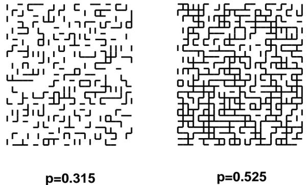
FIG. 11. Illustration of bond percolation in 2D. The nodes are placed on a  $25 \times 25$  square lattice, and two nodes are connected by an edge with probability  $p$ . For  $p = 0.315$  (left), which is below the percolation threshold  $p_c = 0.5$ , the connected nodes form isolated clusters. For  $p = 0.525$  (right), which is above the percolation threshold, the largest cluster percolates.
