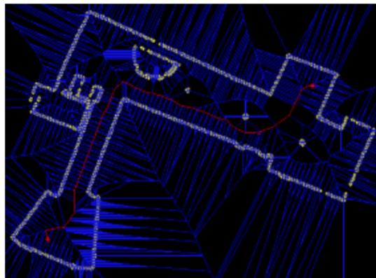
Figure: Driving path (red), and obstacles detected (white).
