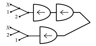
Figure 9: The first half of the squaring gate. The final merging on the right side represents an ordinary voting tree comparison between the outputs of the top and bottom chain of gates.
