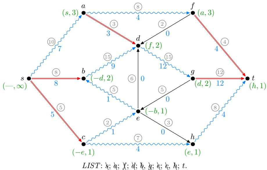
The node  $t$  received a label, which means that the current flow is not optimal. By following the labels backward from  $t$ , we discover the augmenting path  $s-a-f-d-b-e-h-t$ . We augment the flow along this path by 1, bearing in mind that the path traverses the arcs  $(b, d)$  and  $(e, b)$  in the backward direction, so augmenting the flow along the path involves *decreasing* the flow on these arcs. This results in the following flow.
