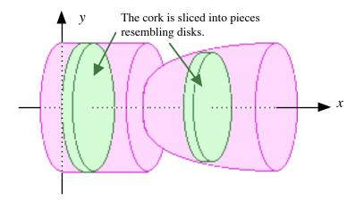
**1.(c)** The portion of the champagne cork nearest the *y*-axis is a cylinder with a radius of 1.5cm and a height of 2cm. The volume of this portion of the cork (in cubic centimeters) is given by:
