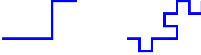
Figure 4.3: Bumping a shortest path at indices 2, 6, 9
