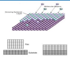
Etero-epitaxy: different lattice parameters between substrate and film crystals
