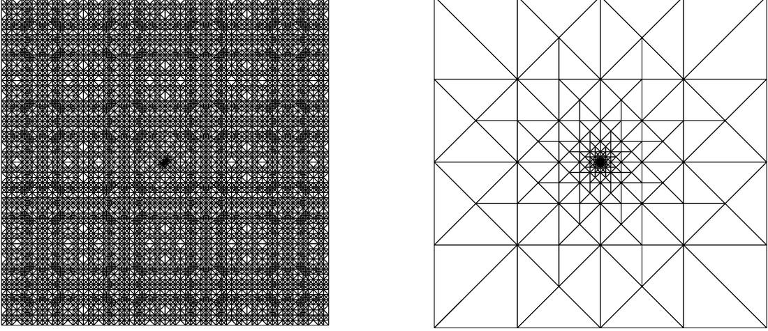
FIGURE 4.2. Refined mesh after  $k = 15$  iterations for the AFEM MNS of Morin-Nochetto-Siebert of Lecture 2 (left: 8077 degrees of freedom) and by the new AFEM (right: 363 degrees of freedom) with  $\theta_E = \theta_0 = 0.4$ . It is quite evident that Marking Strategy O yields a suboptimal performance in terms of degrees of freedom.
