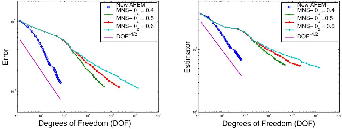
FIGURE 4.3. Decay rates of error (left) and estimator (right) for the new AFEM vs the AFEM MNS of Morin-Nochetto-Siebert of Lecture 2 for several values of parameter  $\theta_0 = 0.4, 0.5, 0.6$  and  $\theta_E = 0.4$ . As the marking parameter  $\theta_0$  increases from 0.4 to 0.6 the curve flattens out thereby showing lack of optimality and its sensitivity to  $\theta_0$ . On the other hand, the new marking exhibits optimal decay.
