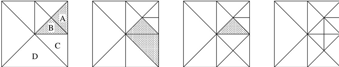
FIGURE 4.1. Recursive bisection refinement: Triangles A, B are initially marked for refinement. Triangle B yields a concatenation of refinements that stops in triangle D.
