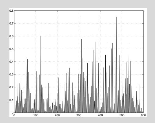
Dissipation-range intermittency from wind tunnel turbulence where hot wire anemometry has been used to measure the longitudinal velocity derivative at a single point (D. Hurst & J. C. Vassilicos). The horizontal axis spans 8 integral time scales with  $Re_{\lambda} \sim 200$ .
