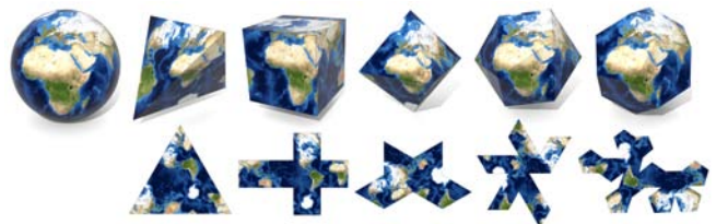
Fig. 2. A conformal cone parameterization is equivalent to flattening a smooth surface, like the sphere, over a polyhedron, which can then be cut and unfolded into the plane without further distortion. By adding more and more cone points, one can make area distortion arbitrarily small. (Texture courtesy NASA Earth Observatory.)
