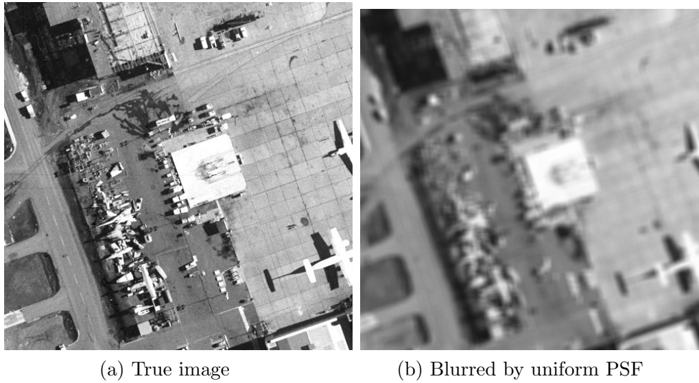
Figure 3. (a) The true “Airfield” image \mathbf{f} of size 500 \times 500 . (b) The observed image \mathbf{g} = \mathcal{T}\mathbf{f} + \mathbf{n} , where \mathcal{T} is defined by the 11 \times 11 uniform PSF \mathbf{k} as in (2) and \mathbf{n} is Gaussian noise defined in (36). The size of \mathbf{g} is of 490 \times 490 pixels.
