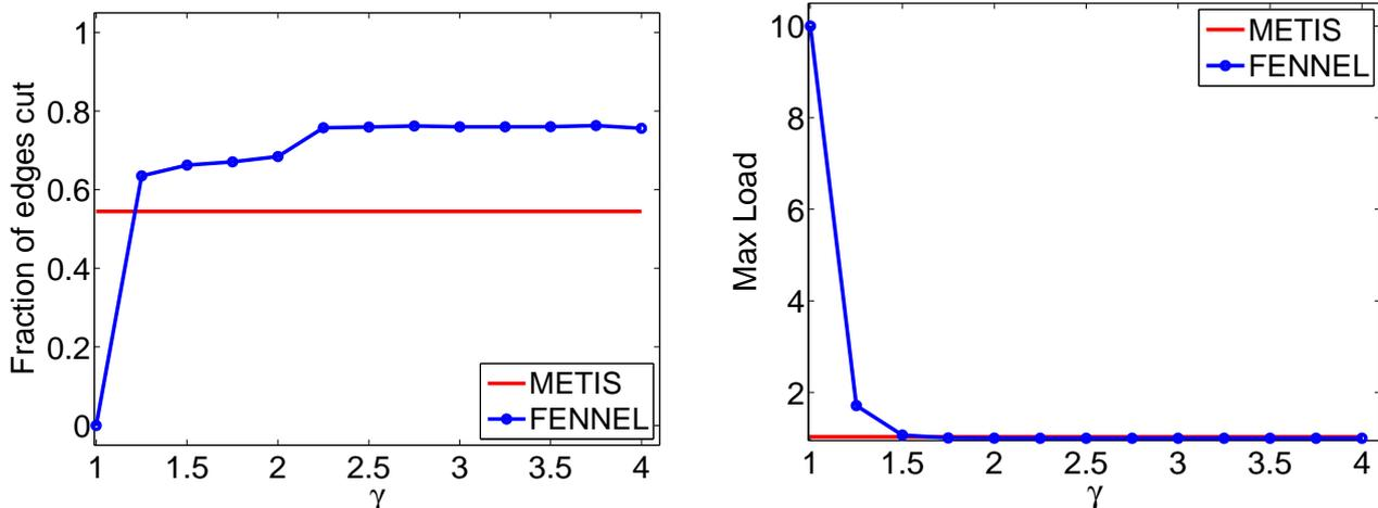
Figure 1: Fraction of edges cut  $\lambda$  and maximum load normalized  $\rho$  as a function of  $\gamma$ , ranging from 1 to 4 with a step of 0.25, over five randomly generated power law graphs with slope 2.5. The straight lines show the performance of METIS.
